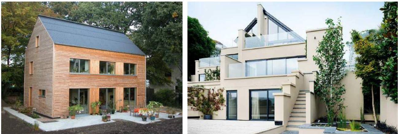
**Figure 3** Two contrasting designs for a domestic property. The one on the right would be far more challenging to make airtight.
