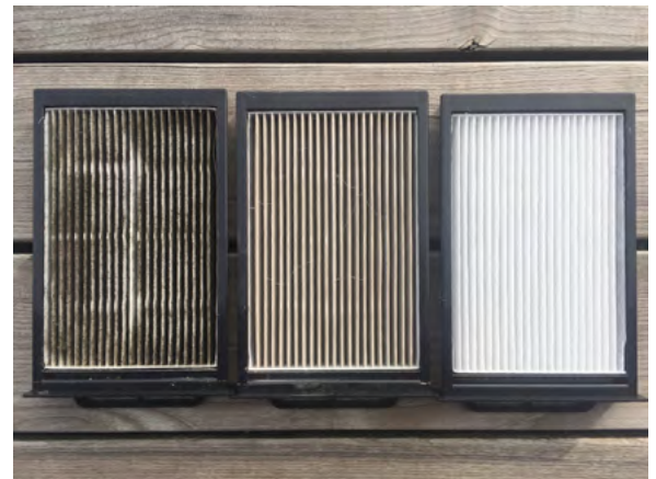
Old and new MVHR filters – left to right: intake; exhaust; new. Image: George Mikurcik
